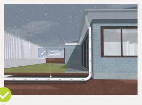
So water can drain away from your slab, ensure there is a sealed path installed around
